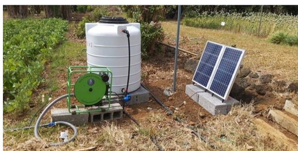
Figure 23: SF-2 Futurepump solar power-driven pump with drip irrigation
