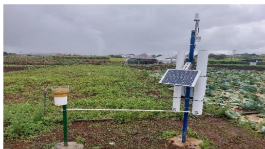
Figure 27: The Cosmic Ray Neutron Sensor at Plaine des Papayes
